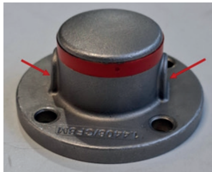
Two lateral sprues on the top of the cap
