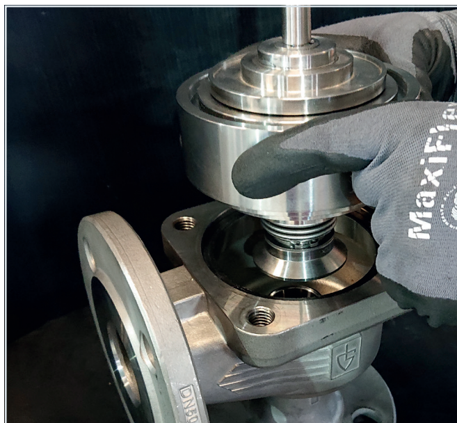
7.15 Carefully place the spindle assembly with the assembled plug assembly onto the screwed-in seat.
