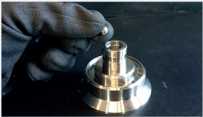
4.10 Coat the base of the cone bore with a little stainless steel grease and insert the ball.
