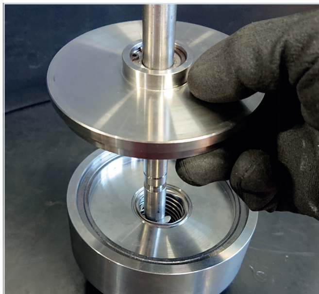
7.13 Fit guide plate and spring plate on the spindle.
