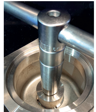
Screwing seat into body.
