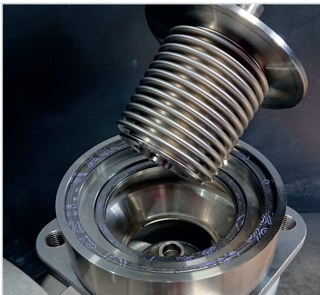
7.11 Insert the spindle into the bellows assembly.
