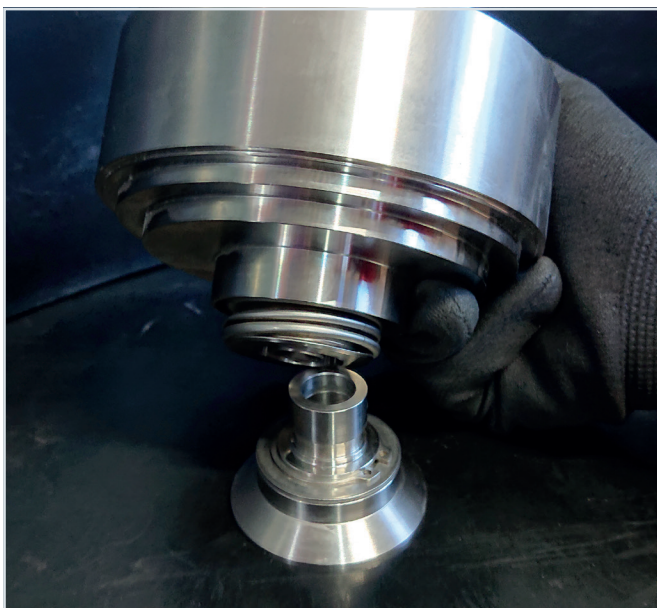
7.14 Insert the spindle into the cone with the greased ball inserted.
