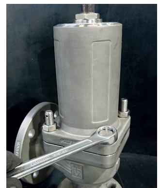
Screw connection of spring housing and body.
