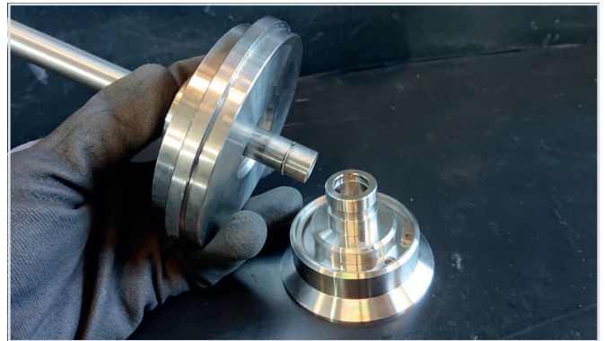
4.12 Insert the spindle into the cone.
