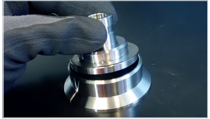
4.8 Insert the cone and shim discs.
