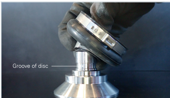
5.11 Insert the ear clamps into the outer groove of the elastomer bellows.
